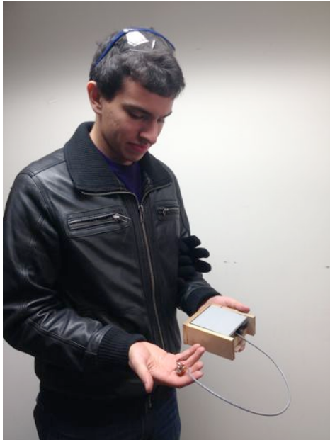
Figure 3. Noah Fishman’s “trigger instrument”, a compact design made from wood and foam rubber and tapped with the fingers.
